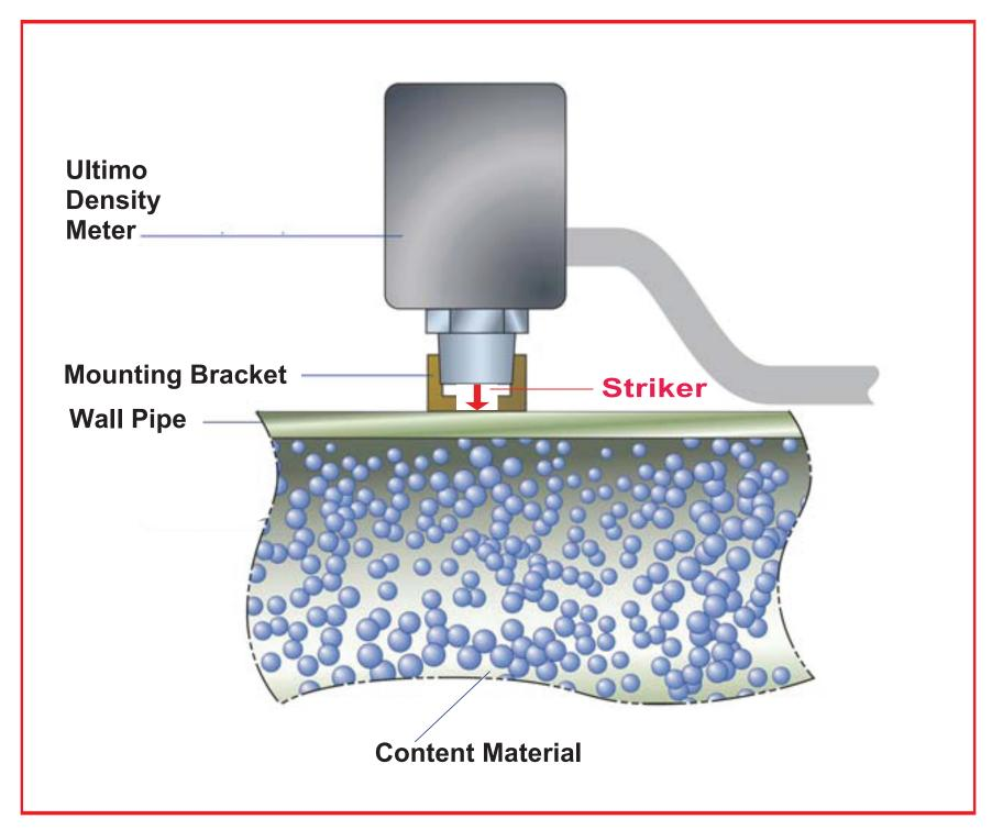
**Ultimo Principle of Operation Diagram**
